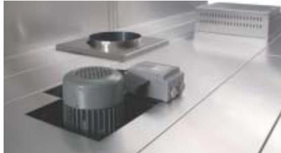
*Fan motor for air turbulence.*
