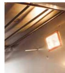
The light in deck ovens with an insulated door is turned off when the door is closed, ensuring that it is never lit unnecessarily. A small, but important energy-saving measure.
